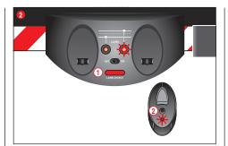
To bond the second controller, press twice on the button "Lane choice" (1). The right LED now lights continuously. Now press the "Bonding button" (2) of the second hand controller. If bonding is successful, both LEDs will then light continuously. The controller is now bonded to the connector track and controls the car on the
