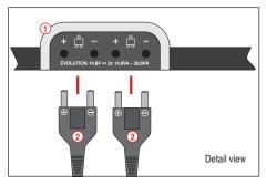
Connect the two plugs 2 on the transformer with the connection sockets 1 on the connector track, **taking care not to reverse the** polarity of the plugs and sockets!
